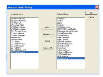
Verification reports can be customized by the user utilizing the Measured Grades Setting window.
