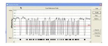
The SRP illustrates the bars and spaces in the code. The red line represents the Global Threshold. The peaks above the Global Threshold indicate spaces and the peaks below the Global Threshold indicate bars. The bottom of the SRP window recreates the barcode based on the digital values displayed in the graph.
