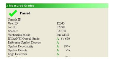
The Measured Grades window displays the verification parameters reported by the Xaminer Elite verifier. This window displays analysis results for the active record. Typically, this is the most recently scanned or uploaded record; however, it may be any selected record from the active SVS file.
